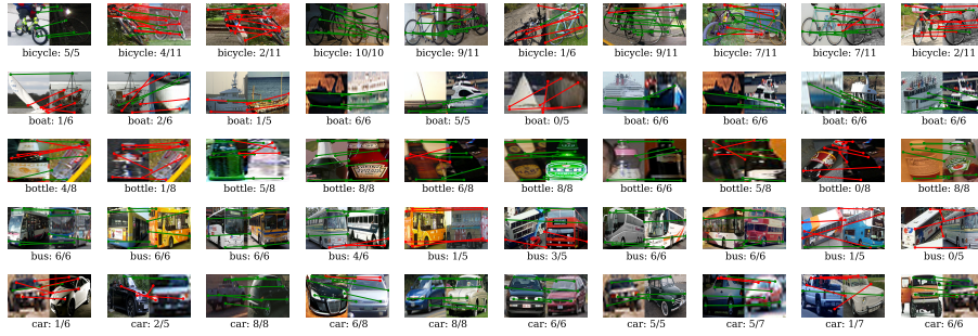
Fig. 5. Illustration of the matching results by SCGM combined with BBGM on the Pascal VOC. Green and red lines represent correct and incorrect node matchings respectively. The subtitle of each figure shows the correct matched/total keypoints count.
